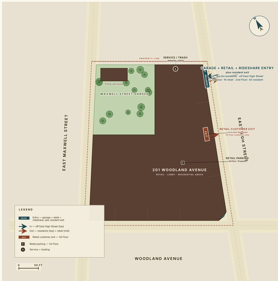
FIG. 12.1 Vehicular access at 201 Woodland Avenue. Garage cars, retail customers, and rideshare drop-offs enter through a drive at the north end of the East High Street frontage. Residents come back out the same drive. The 1st Floor, set behind the retail facade, holds 10 spaces for retail customers; the ramp climbs to a 2nd Floor deck holding 43 resident spaces. Retail customers exit one-way through a separate door at mid-East High — so retail in-traffic and out-traffic never share a door. Service and trash collection occur at the north end of the building.
