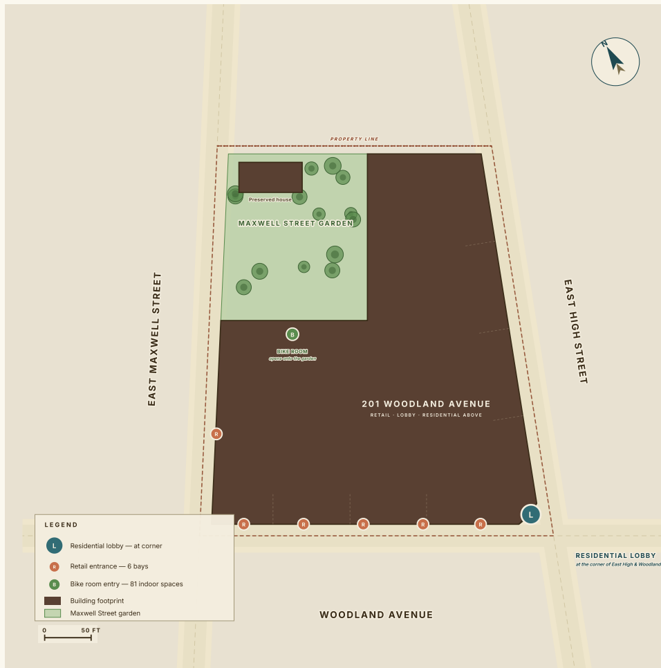
FIG. 11.1 Pedestrian entrances at 201 Woodland Avenue. The residential lobby is at the prominent corner of Woodland & East High. Six retail bays open along Woodland Avenue and East Maxwell Street. Bike storage is tucked at the back of the building, opening directly onto the Maxwell Street garden.
